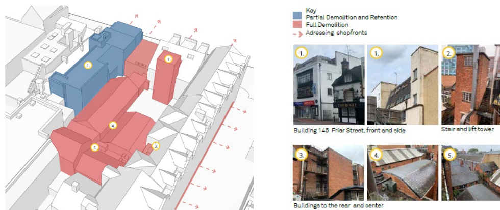
Figure 8 - External demolition work - aerial view and related photographs
